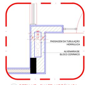
**2 DETALHE - SHAFT HIDRÁULICA**
